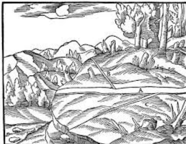
A—Vein. B—Folds incised from the surface of the hangingwall. C—Same from the footwall.
